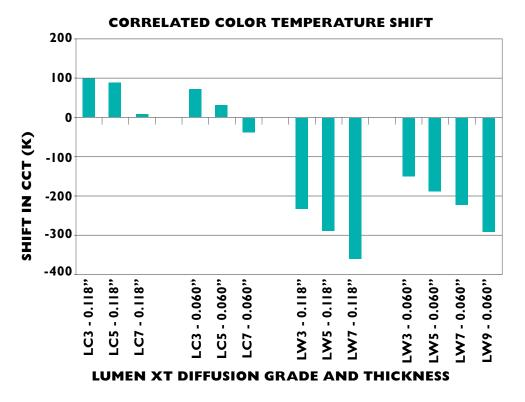
This graph shows measured shifts in Correlated Color Temperature (CCT) of light from an LED light fixture with a diffuser sheet vs. the same LED fixture without a diffuser. The LED fixture's CCT without a diffuser is 6000 K.
