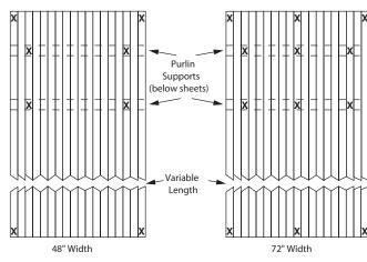
48 inch wide sheets shouldbefastenedtosup ports at all four corners, and at points 6" in from the edges of each purlin support.
