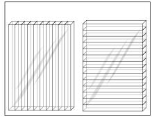
Extruded ribs shall be installed in a vertical direction for drainage.
