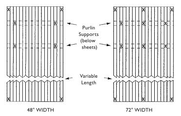
48 inch wide sheets should be fastened to supports at all four corners, and at points 6" in from the edges of each purlin support.
