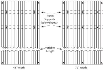
48 inch wide sheets shouldbefastenedtosup ports at all four corners, and at points 6" in from the edges of each purlin support. 72inchwidesheetsshould be fastened to supports at all four corners, and at points6"infromtheedges of each purlin support and in the center of the purlin supports.
